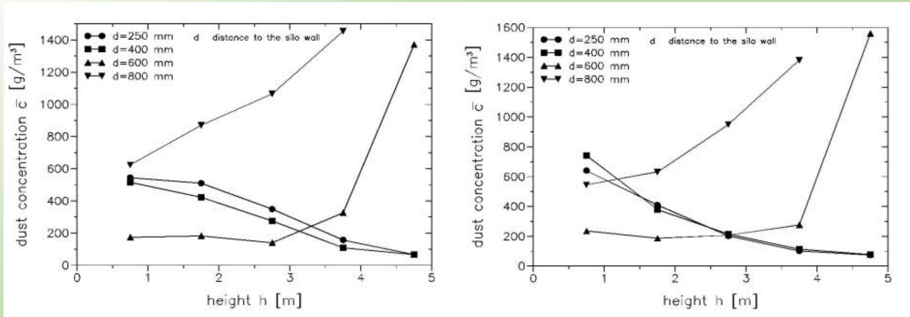
Solid fed pneumatically via a vertical nozzle at the centre of the top of 12 m<sup>3</sup> silo. With no solid in the hopper in the left-hand graph and with solid in the hopper in the right-hand graph.
