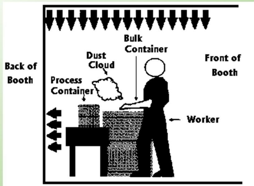
Frequently the process container is stood on a weigh scale
