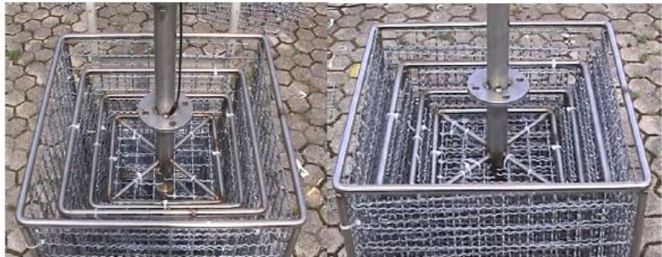
Figure 1: Assembly of the cube. System of grids 40 x 4 mm with 4 layers (left) and 12 layers (right)
