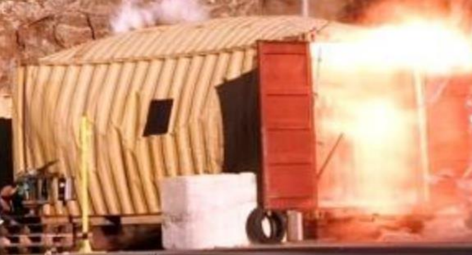
Venting through door
