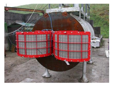
4 m<sup>3</sup> explosion test vessel with two 0.2 m<sup>2</sup> rectangular CV explosion vent panels and flameless venting devices
