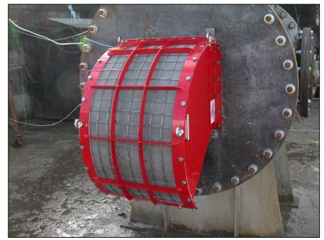
2 m<sup>3</sup> explosion test vessel with rectangular CV explosion vent panel
