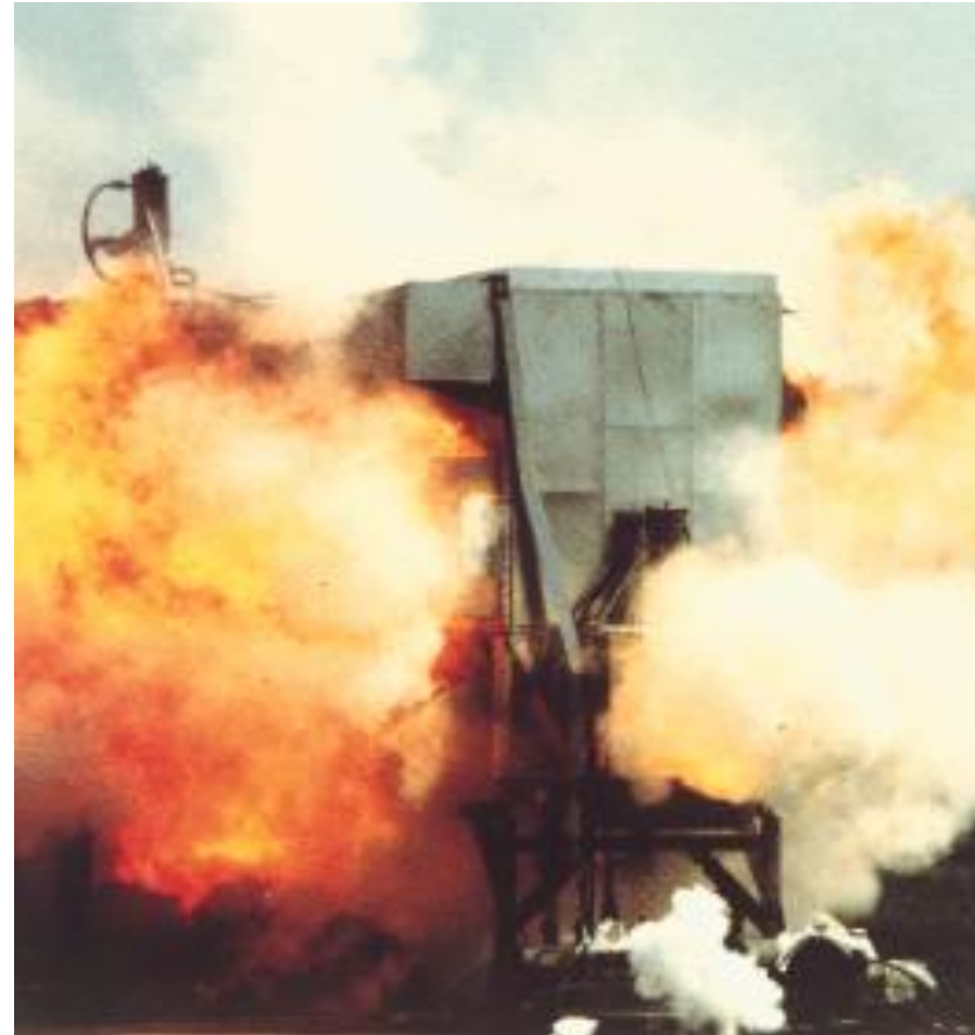
A dust explosion test in large scale facility [2]
