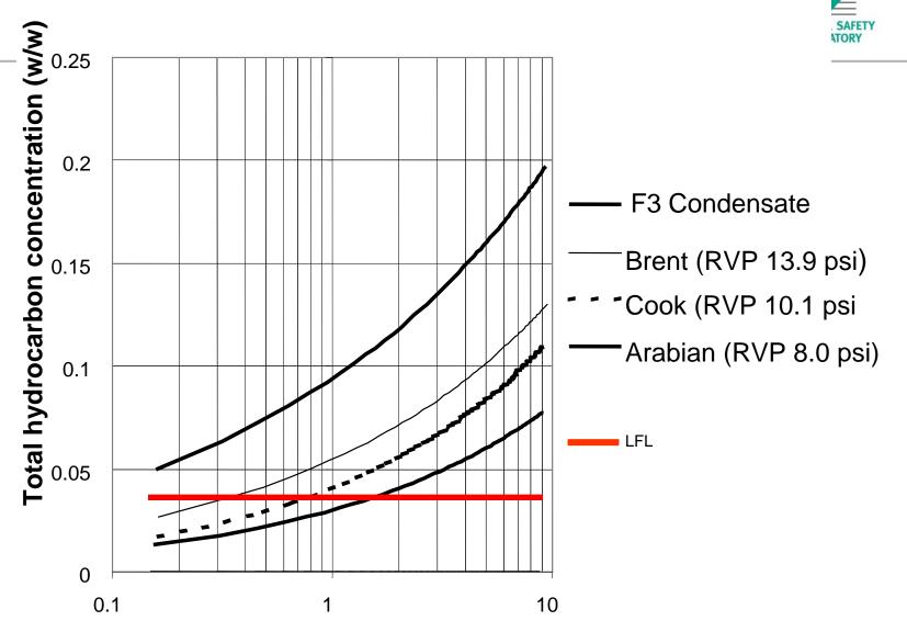
Mass release per metre of (total) tank perimeter (kg/s/m)
