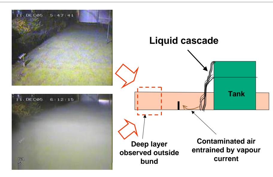
Even when a deep layer accumulates around the tank the vapour flow entrains some fresh air
