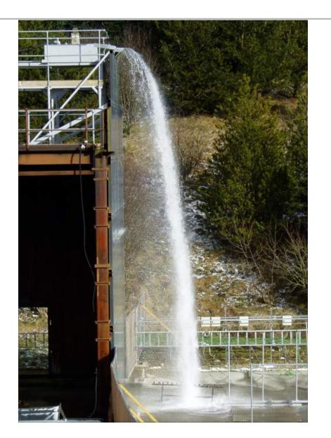
Measurements of liquid and vapour temperatures in full scale experimental cascades. Near field dispersion: Is entrainment of air suppressed by the deep accumulating vapour cloud ?
