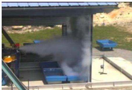
Impinging two-phase jet – from the INERIS test series report
