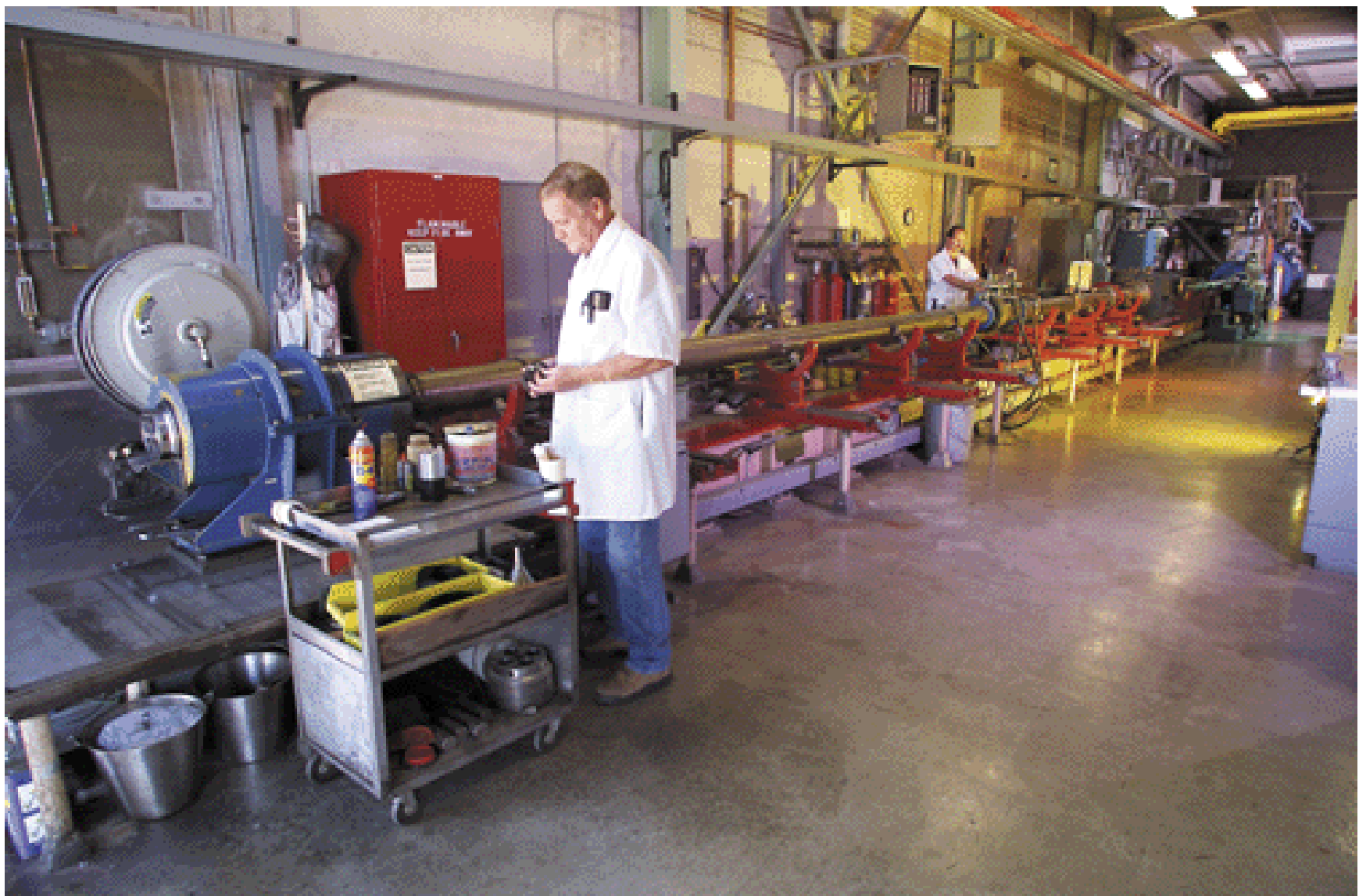
Livermore's largest two-stage gas gun is 20 meters long. Its projectile flies down the barrel at speeds up to 8 kilometers per second to produce a shock wave millions of times the pressure of air at the surface of Earth. Technicians Leon Raper (left) and Keith Stickle are setting up the gas gun for an experiment.
