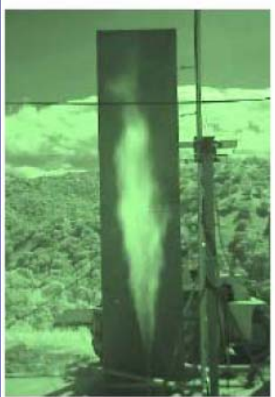
Vertical Flame 10-12 ft tall, 2-3 ft wide (H 2 flame at SRI test site)
