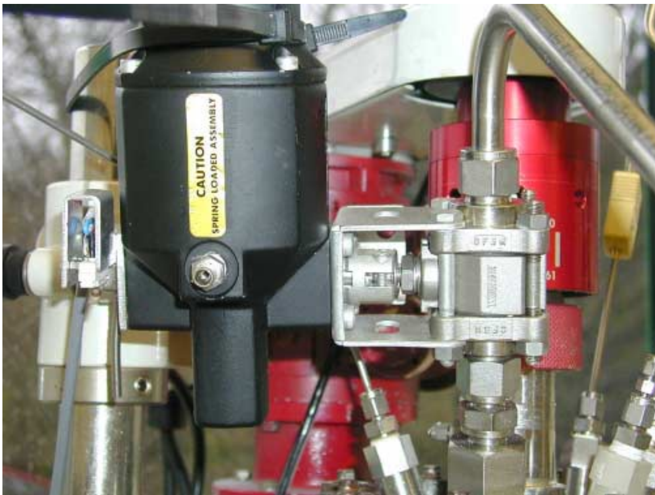
Pneumatically actuated ball valve, micro switch and nozzle holder
