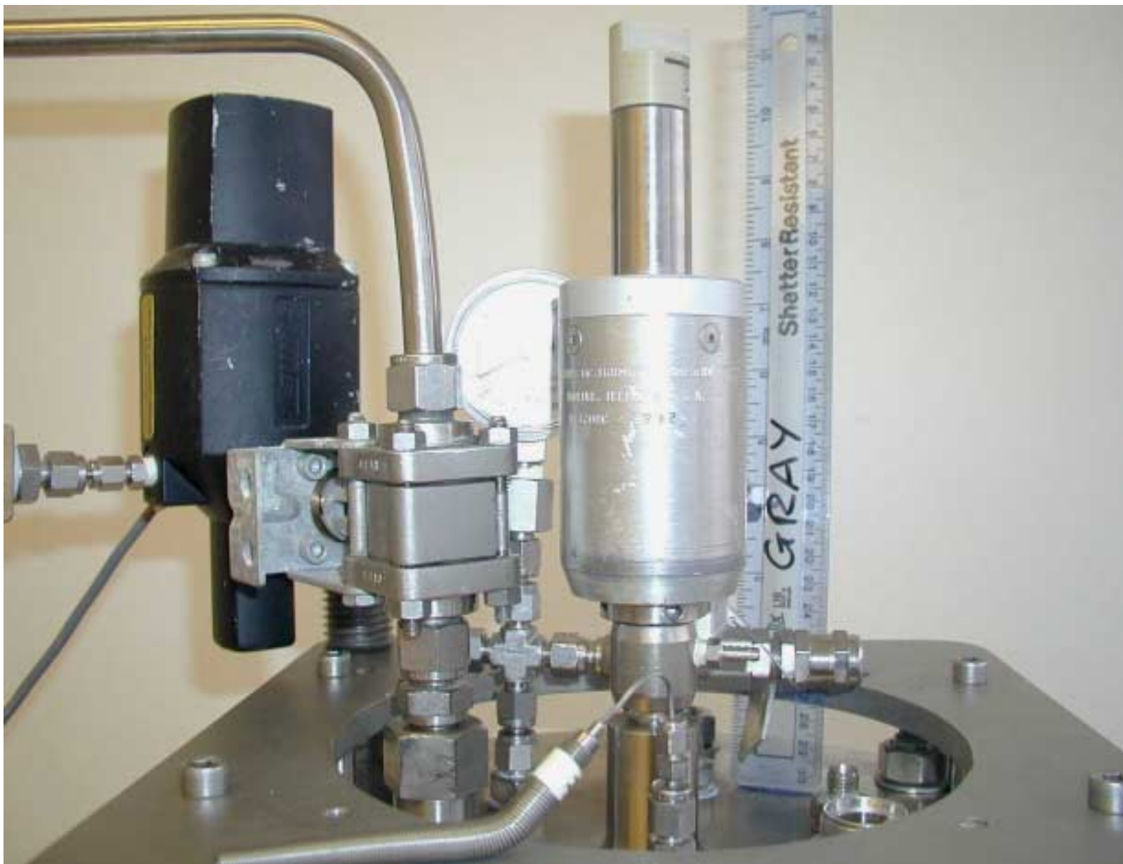
Magnetic drive, pneumatically actuated ball valve, pressure relief valve, nozzle holder
